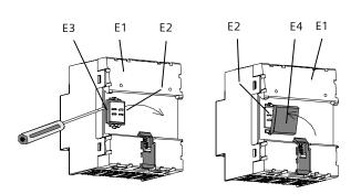
Figure 4: Covering the contact system
