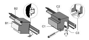
Figure 2: Installing / dismantling the device
