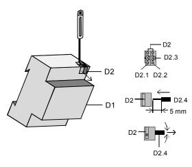
Figure 3: Attaching / removing the bus terminal
