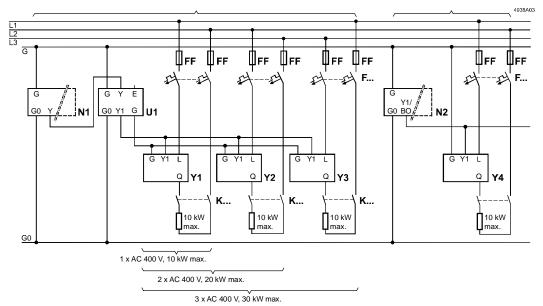
Connection diagram 3 (standard circuit)
