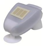
The AP 257/22 weather station (GPS) contains all sensors, electronic systems for weather data analysis and the bus coupler in one compact enclosure. It measures wind speed, brightness and temperature, detects dusk / dawn and precipitation and receives the GPS signal for date and time.
