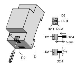
figure 4: Connecting and disconnecting bus wires
