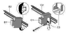
figure 3: Mounting and unmounting a DIN rail mounted device
